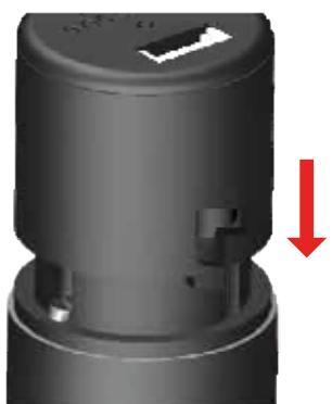
Align the housing to the base plate and slide it over the latter
