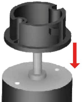
Align the base plate to the motor shaft using the centering tool
