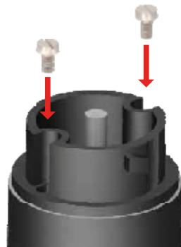
Then fix the base plate to the motor flange using two screws
